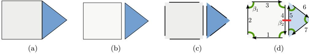
Figure 1: Combinatorial maps: construction by successive decompositions. (a) Original image; (b) Decomposed faces; (c) Decomposed edges; (d) 2-Map: arrows represent darts,  $\beta_1$  and  $\beta_2$  operators are respectively represented by arcs and segments.
