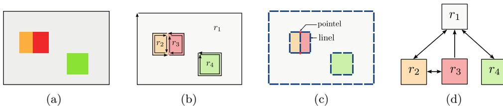
Figure 2: Combinatorial maps: construction by successive decompositions. (a) Original image; (b) Combinatorial map for topology: the image contains four regions  $r_i, i \in \{1, 2, 3, 4\}$ ; (c) Interpixel matrix for geometry: pointels and linels are represented by bold circles and segments and correspond to the embedding of the darts; (d) Tree of regions for inclusion relationships:  $r_1$  contains  $r_2, r_3$  and  $r_4$ .  $r_2$  and  $r_3$  are adjacent.
