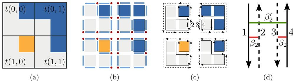
Figure 4: Topological tile. (a) An image divided into 4 tiles; (b) Geometrical representation; (c) Topological representation.  $\beta_2'$  operator is represented by bold segments; (d) Detail of the connection between  $t(0,0)$  and  $t(0,1)$ . Darts 2 and 3 belong to the infinite region.  $\beta_2(1) = 2$ ,  $\beta_2(4) = 3$ ,  $\beta_2'(1) = 4$ .
